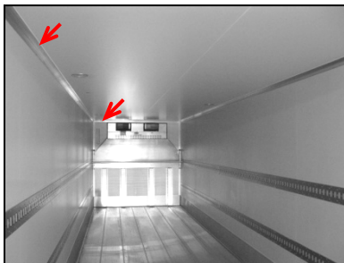
General view inside (adhesives)
